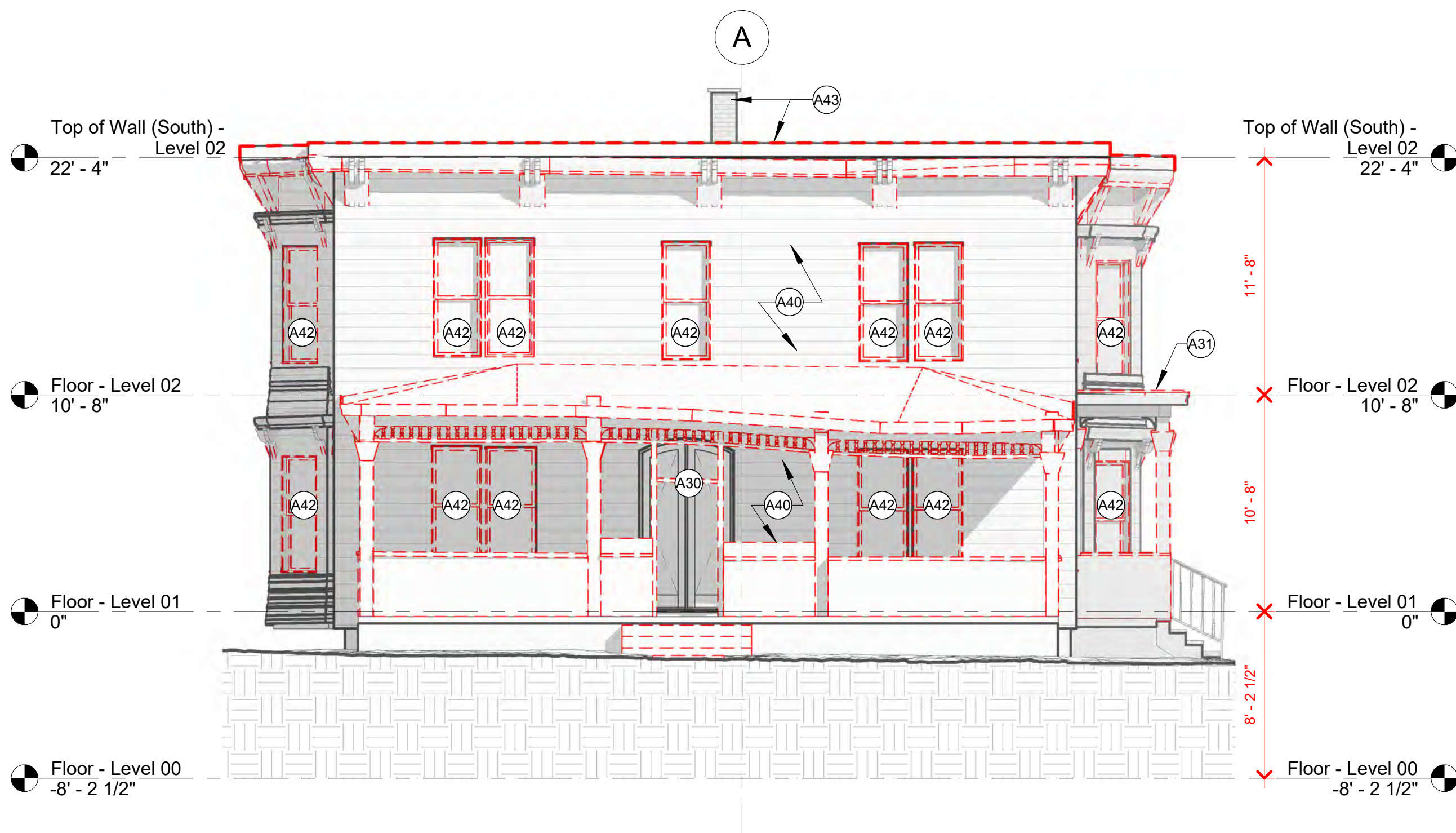
3 Building Elevation - South Demolition 3/16" = 1'-0"
