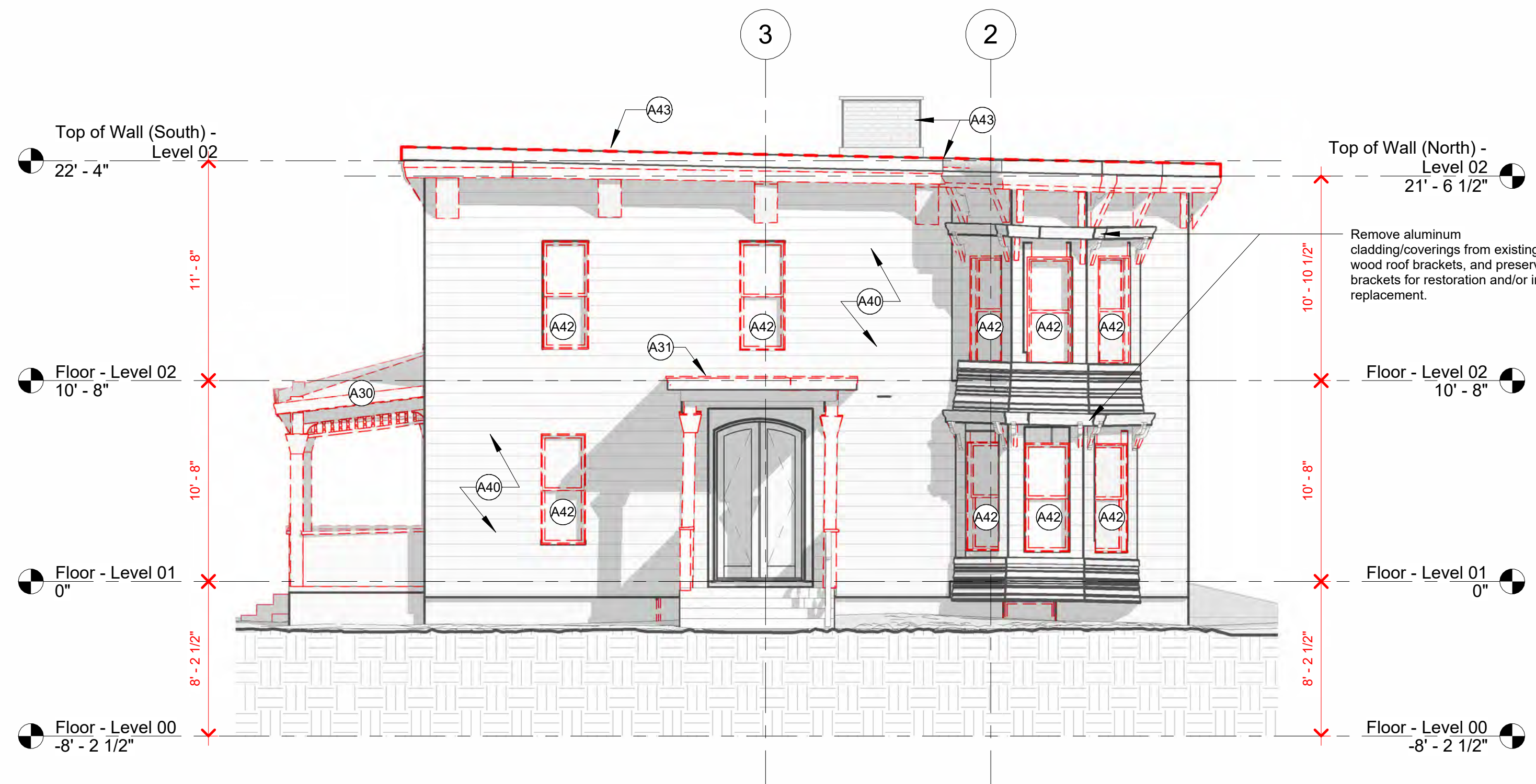
2 Building Elevation - East Demolition 3/16" = 1'-0"
